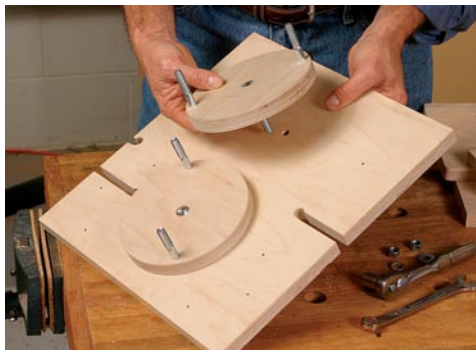
Attach the circles. With outside bolts in place, secure the circles to the front plate with 3/8-in. bolts through the center holes. Hand-tighten double nuts over the washers and lock the nuts.
