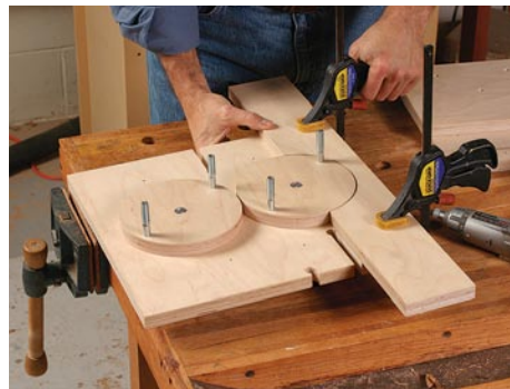
Attach the top faceplate. Align its top edge with that of the front plate. Clamp it in place, and attach with screws from the rear.
