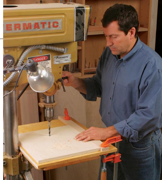
Locate the circles on the front plate. Drill two 3/8-in. holes on the centerline for the circles' center holes. Use a fence to ensure that the holes are aligned.
