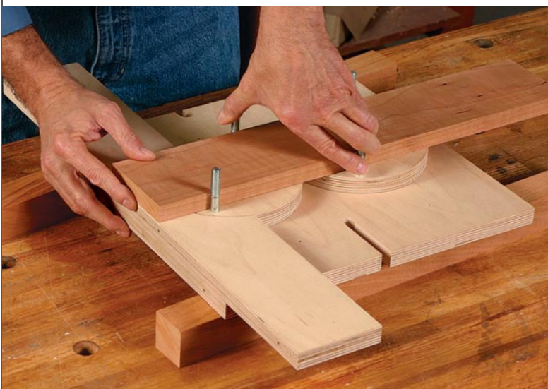
Attach the circles. With outside bolts in place, secure the circles to the front plate with 3/8-in. bolts through the center holes. Hand-tighten double nuts over the washers and lock the nuts.
